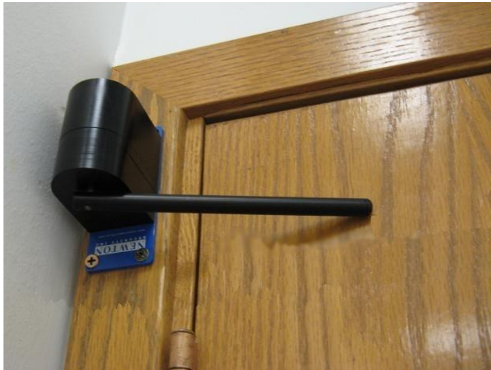
Figure 39 –Position of Encoder (Public door only)
