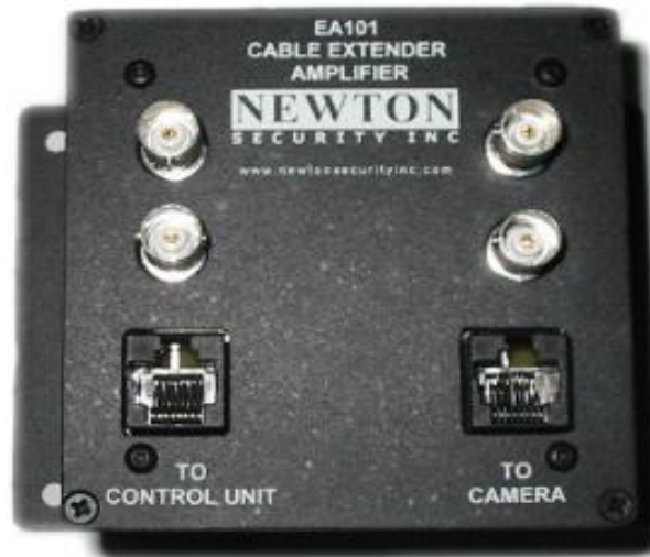
Figure 9 – T-DAR Cable Extender/Amplifier
