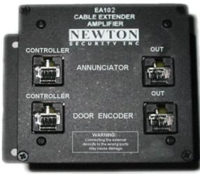
Figure 12b – T-DAR Encoder Cable Extender
