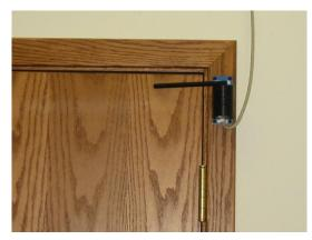
Figure 39 – Position of Encoder on door
