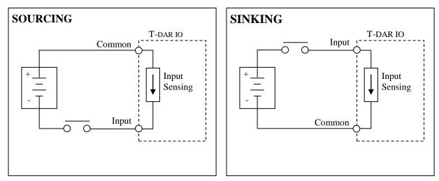
Figure 40 - Sourcing/Sinking Inputs
