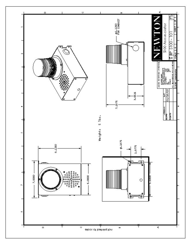
Figure 4 - T-DAR Annunciator CAD
