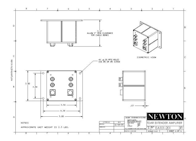
Figure 10 – T-DAR Cable Extender/Amplifier CAD
