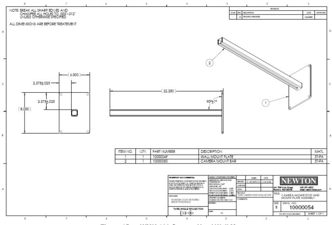
Figure 15a – WMK-100 Camera Head Wall Mount
