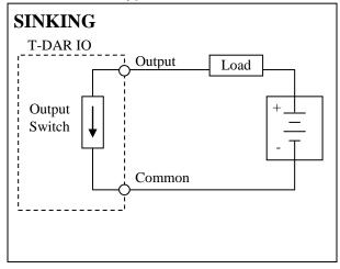
Figure 41- Sinking Outputs
